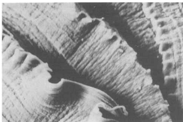
FIGURE 12 SEM of fracture surface for the blend D at (400X)
